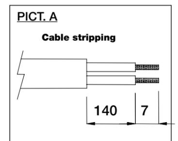
4. Connect the individual conductors to the terminal of the bracket (5) paying attention to respect the polarities and the insulation class of the luminaire.
